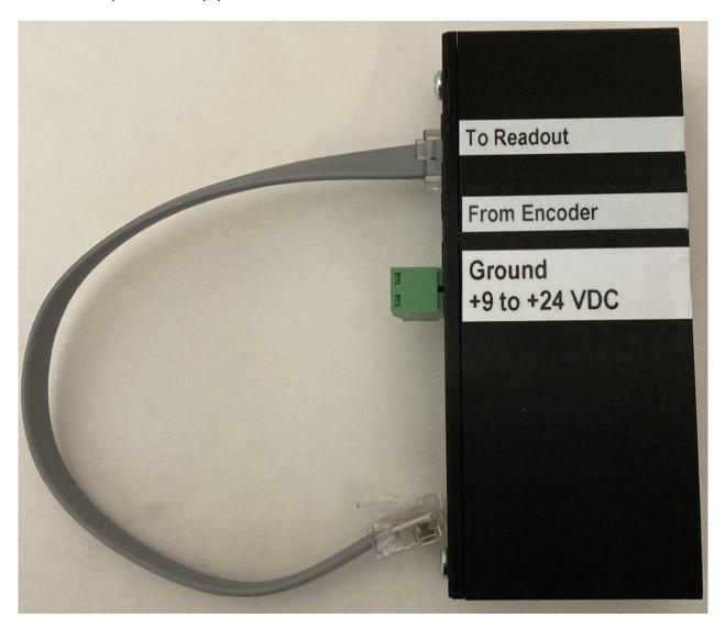
Plug the encoder into the EPS. The EPS is then plugged into a readout via a 6-Pin connector cable (provided with the EPS). After fully charging (4–5 hours), the EPS provides power to the encoder for 6+ months. For the EPS to fully charge, +9 to +24 VDC must be applied as labeled on the unit.
