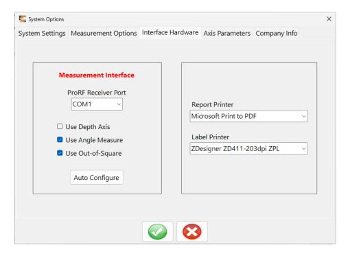
The Measurement Interface is used to configure the ProScale measurement equipment. The system supports the ProRF Universal receiver, with ProRF Encoder Transmitters on each measuring gage.
