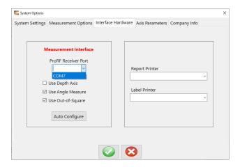
10. Enable the Angle, Out-of-Square, and/or Depth Axis, as appropriate.
