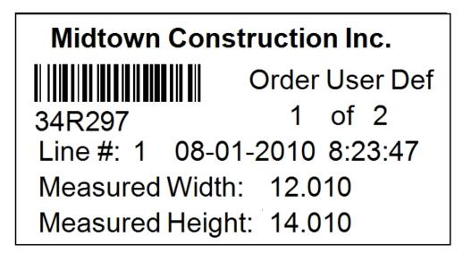
ProCAB QC supports an optional label printer that can be used to print labels containing part measurement data. The part label is fully user configurable via the Reports Manager configuration tool. See <u>Configuring Printing Templates</u> for more information regarding this feature.
