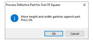
Place the defective part on the ProTable-CAB and move the gantries against the sides of the part. Press the OK button to allow the system to find the line item that matches the part. If no matching line item can be found, the system will indicate the error message shown below:
