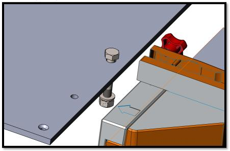
7. Slide the Fence over the M10 bolts, capturing the top of each bolt in the bottom T-slot of the fence profile. After the Fence is in place, and alignment is checked with the saw, tighten all nuts using a 16mm socket/wrench, or with a crescent wrench.
