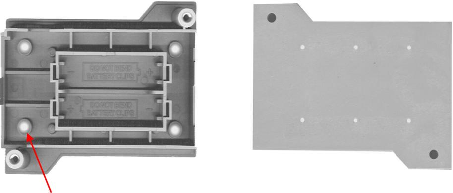
**NOTE: Care must be taken when using the inside holes. If using the lower left hole as shown above, be sure to use a screw that will not rise above the extruded countersink as this may short the input connector.**
