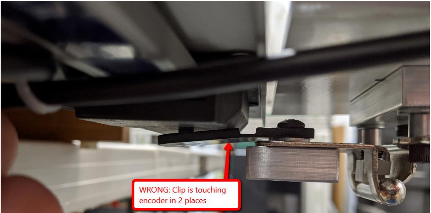
Figure 3: Too much pressure causes the Guide Clip to not engage with encoder properly (View from left end of fence)
