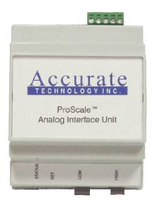
The Analog Interface Unit, or AIU, is an interface device that provides the user of a ProScale measurement system with a method of generating an analog DC output voltage that is proportional to the currently displayed ProScale position. This output can be used with an A/D converter input on a PLC or other device that utilizes an analog input signal.
