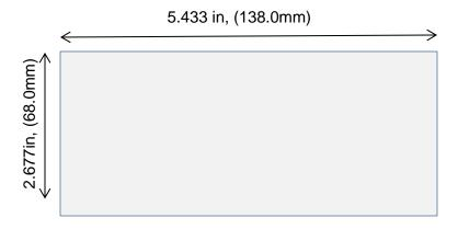
The Readout requires at least 3.35 in (85mm) of depth for adequate installation clearance.
