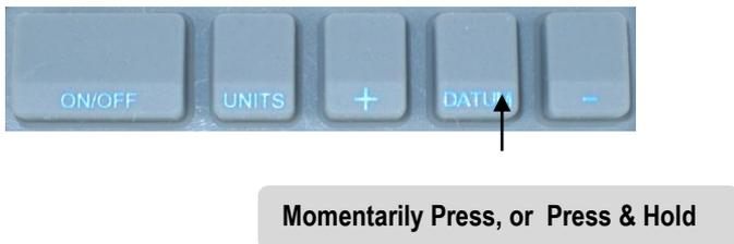
*Momentarily* depressing the **DATUM** key forces the Readout to a user programmed value. This can be zero or any other displayable value. Set the **DATUM** key value by programming [Parameter \(Pr1\)](#).
