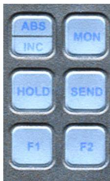
**ABS** Mode – The Display automatically enters ABS mode when power is first applied. This is indicated by the ABS symbol in the upper left corner of the Display. While in the ABS mode, all position measurements are related to the current system reference point. To enter the INC mode, momentarily press the **ABS/INC** button.
