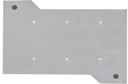
**NOTE:** Care must be taken when using the inside holes. If using the lower left hole as shown above, be sure to use a screw that will not rise above the extruded countersink as this may short the input connector.
