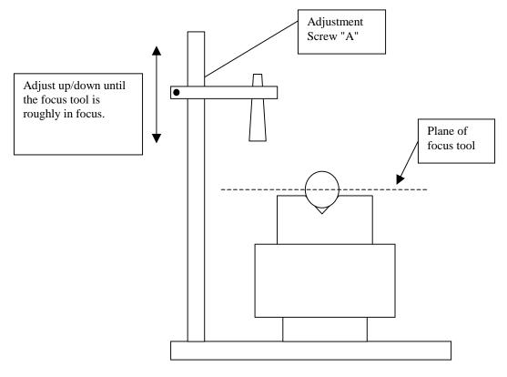
15. Adjust the scope mount's left to right position so the crosshair is parallel to the cutterhead shaft. Tighten the adjustment screw.
