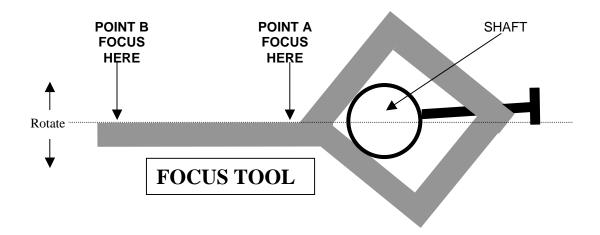
14. Loosen adjustment screw "A" and move the scope assembly up and down on the pole until the focus tool is roughly in focus on the monitor.
