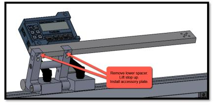
TIP: If you will use multiple add-on plates with your ProStop, you can program OFFSETS in the digital readout so re-calibration is not necessary when the plates are changed (up to 4 offset values can be stored in memory). Offsets are controlled by programming parameters Pr30 to Pr34.
