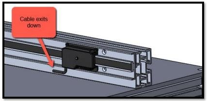
2. Attach the readout bracket to the back of the sliding stop assembly. Tighten bolts.
