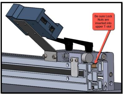
5. Slide the encoder along the electronic scale and position it under the Guide Clip on the Stop Assembly. The post on the top of the Encoder should snap into the slot on the inside of the Guide Clip.
