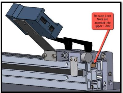
5. Slide the encoder along the electronic scale and position it under the Guide Clip on the Stop Assembly. The post on the top of the Encoder should snap into the slot on the inside of the Guide Clip.
