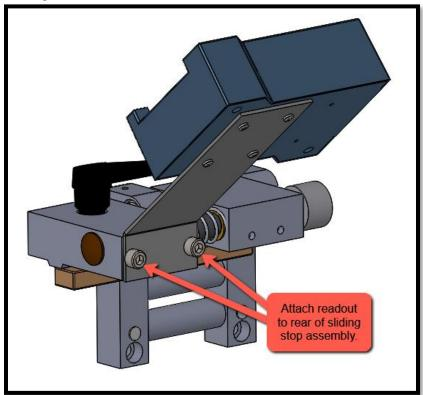
3. Attach the Guide Clip to the back of the sliding stop assembly. Tighten screws. **NOTE: The slot in guide clip faces inward.**
