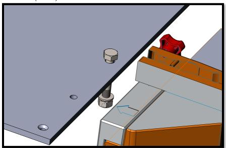
7. Slide the Fence over the M10 bolts, capturing the top of each bolt in the bottom T-slot of the fence profile. After the Fence is in place, and alignment is checked with the saw, tighten all nuts using a 16mm wrench, or with a crescent wrench.
