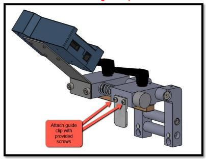
4. Loosen the Stop Assembly lock handle(s) and slide the assembly onto the fence. Be sure to guide the 2 lock nuts into the upper T-slot in the fence.
