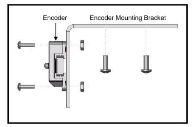
variety of possible mounting surfaces and mounting positions, this step requires you to choose the best screws/nuts to mount the bracket.
