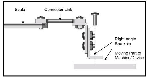
adjusted by loosening the screws, sliding the brackets to the desired length, and re-tightening the screws. One example is shown in the figure above.
