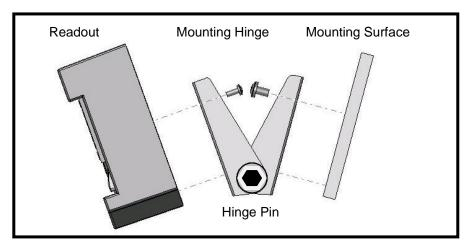
3. Use the Hinge Mounting Screws (8-32 x ¼") to mount the other side of the hinge to the mounting location determined earlier. To adjust the angle of the hinge, loosen the hinge pins with an M5 hexdriver and adjust to the desired angle. Retighten the hinge pins.
