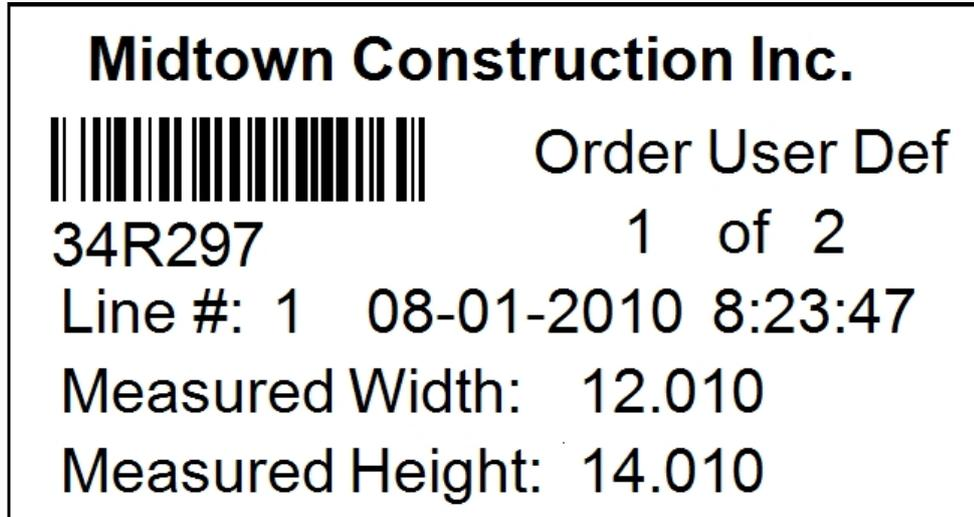
ProCAB QC supports an optional label printer that can be used to print labels containing part measurement data. The part label is fully user configurable via the Reports Manager configuration tool. See Appendix B [Configuring Printing Templates](#) for more information regarding this feature.
