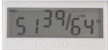
When the measurement is greater than  $99 \frac{63}{64}$  inches, a +100 and/or +200 will illuminate in the upper right portion of the display to indicate this amount must be added to the displayed reading. For example; the LCD pictured above right is indicating a measurement of  $151 \frac{39}{64}$  inches. If the measurement was  $351 \frac{39}{64}$  inches, the +100 and +200 will be illuminated on the display.
