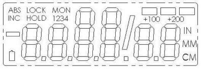
The above figure illustrates all the segments available on the LCD. (Not all segments are used on Digi Readouts)
