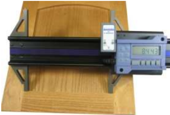
Making an inside measurement. Shown with optional SPC wireless transmitter.
