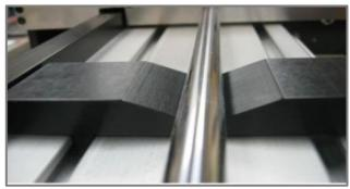
V-blocks ensure rounds and tubular parts are measured the same way by every operator.
