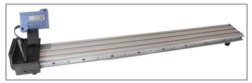
A battery powered readout travels with the moving carriage, and can perform absolute/incremental measurements, send measurements using the built-in SPC port, perform Go/NoGo testing, some statistics on parts being measured, and many more functions.
