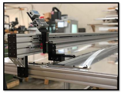
length, width, and squareness comparison), plus a 1.5" steel cone for edge-to-hole measurements<sup>2</sup>. A battery powered readout<sup>3</sup> travels with the moving carriage, and can perform absolute/incremental measurements, store up to 4 offsets (allowing for add-on tooling), send measurements using the built-in SPC port, perform Go/NoGo testing, plus many more functions.
