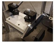
Wear Sheets to protect the table surface. Corner-to-Corner fixtures also shown. Changeover time to length measurement is less than 4 seconds.
