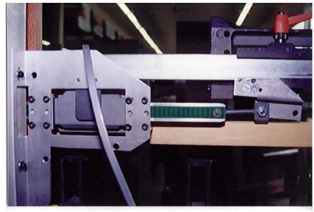
Note how the stop bracket is mounted to the bottom of the sliding stop instead of the top. Also note the readhead bracket is mounted lower on the vertical tube. (The brackets in the photo may be slightly different in shape and color than yours.)
