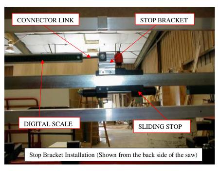
to the stop using two #8-32 x 3/8" flat head screws.
