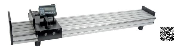
**ProTable** is a single axis battery operated linear dimension measuring system designed for QC/QA functions on the manufacturing floor. It comes with temperature and non-linear error compensation built in.
